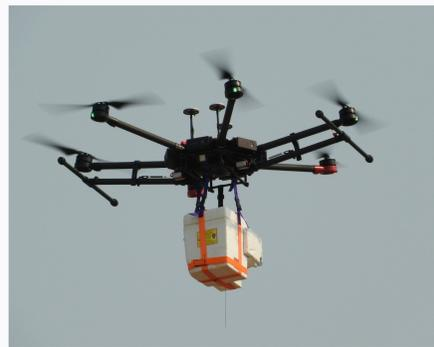
Fig. 1: DJI M600 equipped with an ozonesonde
