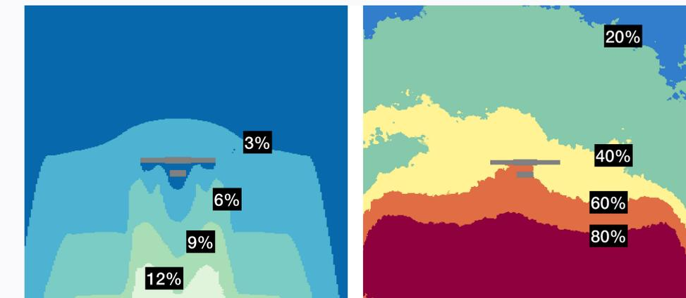
Fig. 6: Relative error map for ascent (left) and descent (right)
