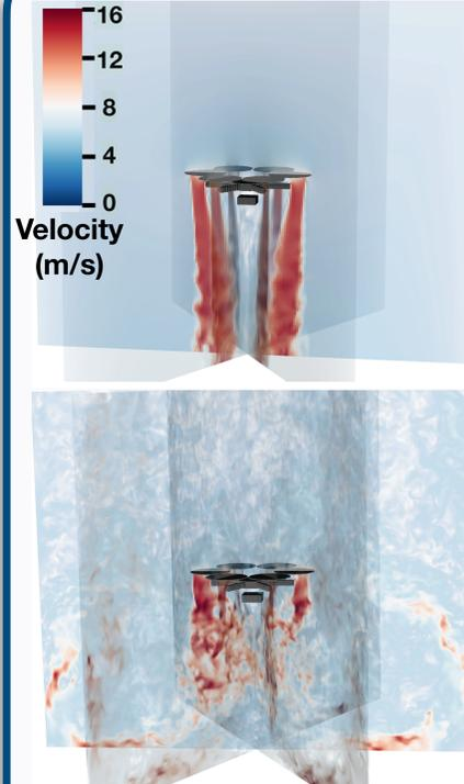
Fig. 3: Airflow (m/s) during ascent (top) and descent (bottom)
