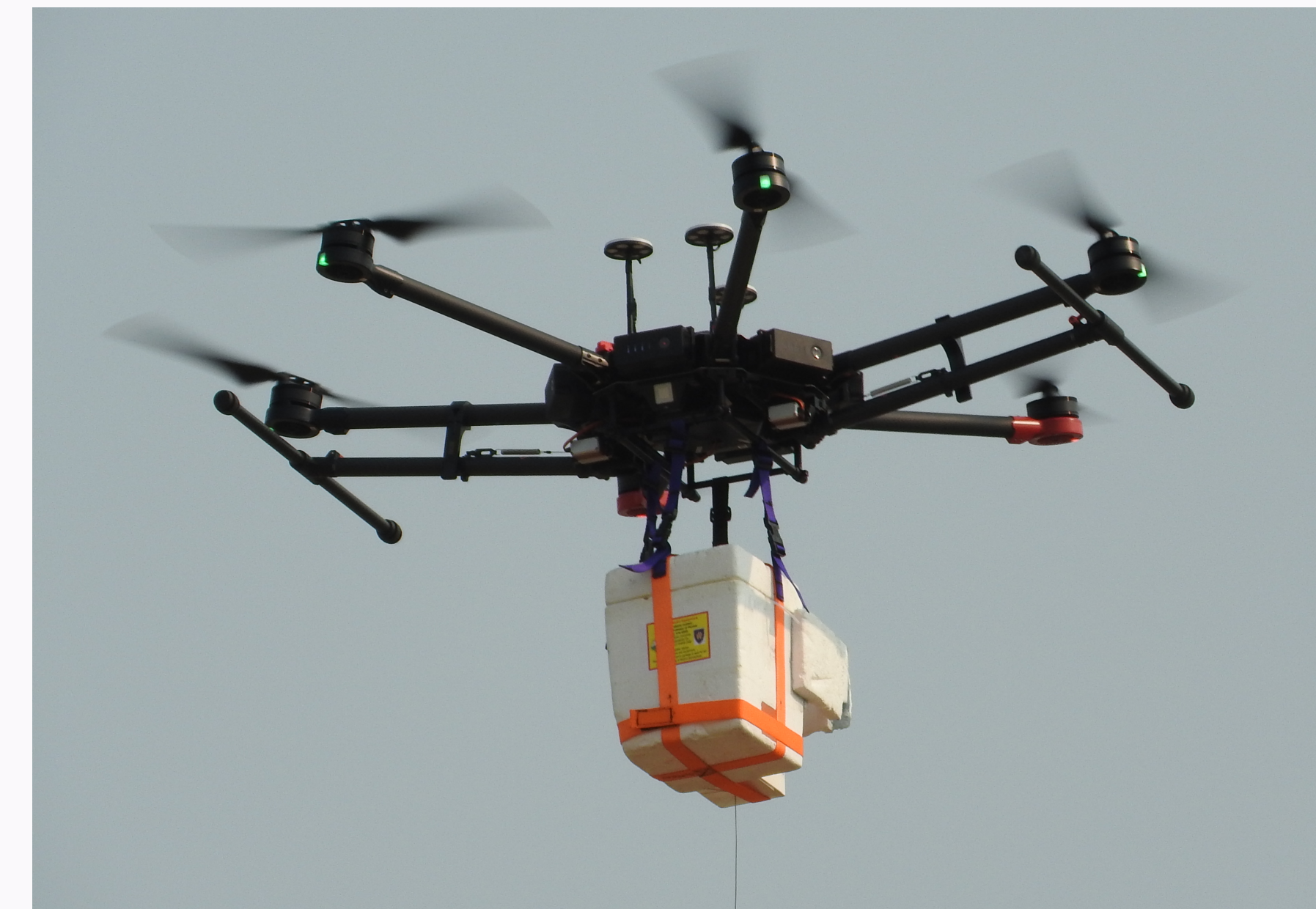
Fig. 2: Drone equipped with an ozonesonde.
