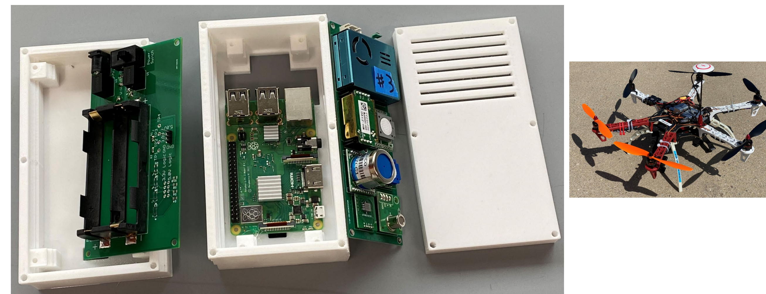
Figure 4. Preliminary assembly will have attachment points added. This will be suspended under a drone (inset) or balloon.
