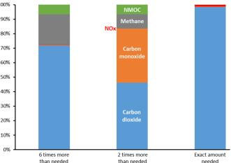
Oxygen level relative to the amount needed to fully combust the fuel
