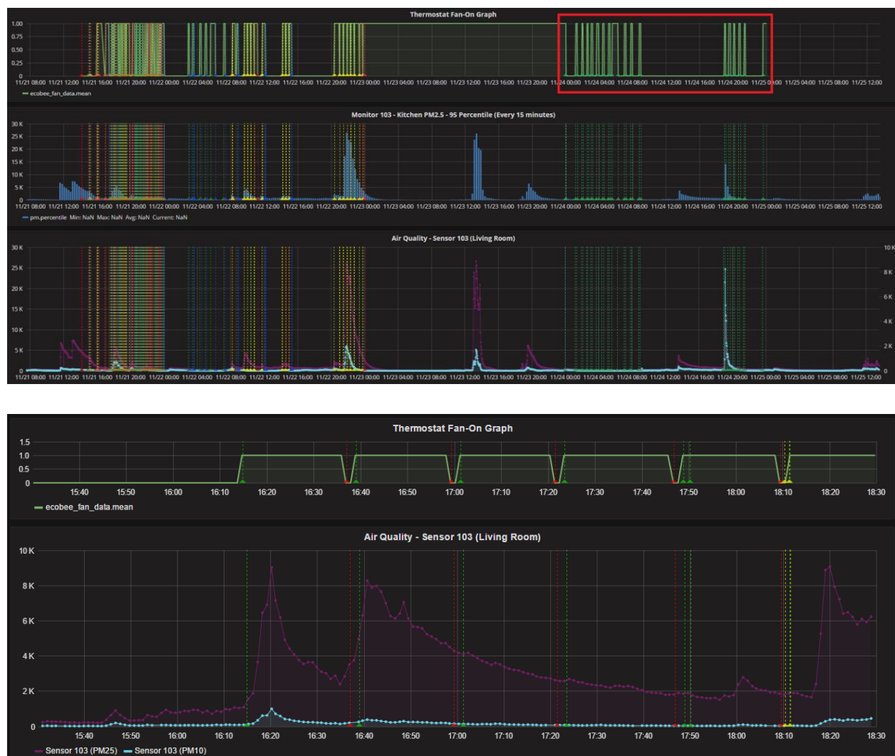
Figure: The graphs show the state of the furnace fan mode and its effects on the small particle (PM2.5) of the indoor air quality. The purple color line graph shows the small particle trend (PM2.5) and the blue color line graph shows the large particle trend (PM10)
