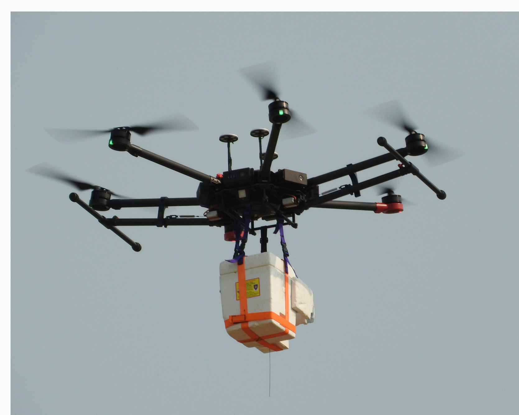
Fig. 1: DJI M600 equipped with an ozonesonde
