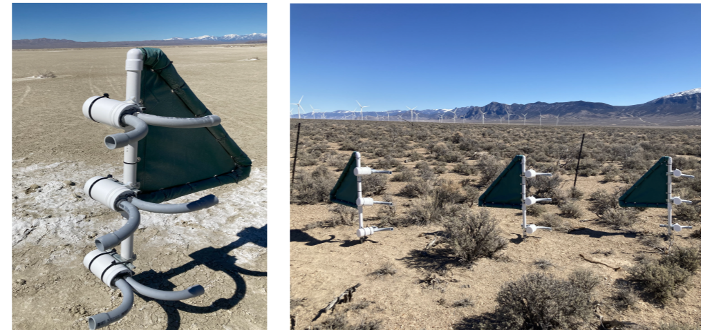
Figure 2. MWAC dust samplers at playa and degraded rangeland sites. Built following guidelines from Blakowski et al. in prep.
